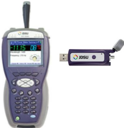
Optical power measurement with the MP-60
